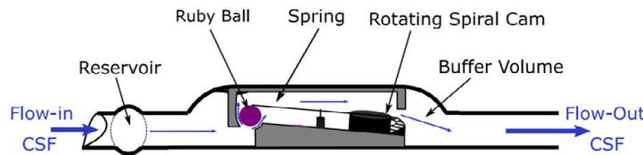
Figure 1: Sketch of a Codman-Hakim shunt valve.
