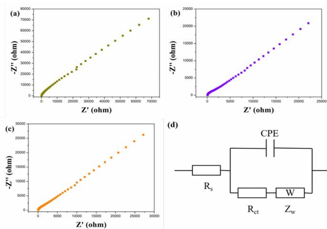
Figure S17: Electrochemical impedance spectroscopy (EIS) of (a) 2IV-based rigid ECD, (b) 2PV-based rigid ECD and (c) 2BV-based rigid ECD and (d) the corresponding analog equivalent circuit.
