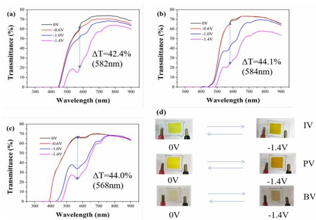
Figure S21: Spectroelectrochemistry of (a) IV-based rigid ECD, (b) PV-based rigid ECD and (c) BV-based rigid ECD under different applied voltages and the image of corresponding devices.
